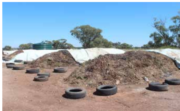
COOLAMON SHIRE'S ORGANICS' FACILITY WITH COVERED WINDROWS, EXPOSED FOR INSPECTION
